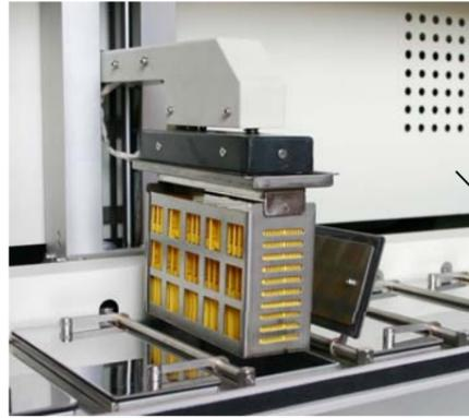
The electromagnetic arm moves the baskets across all processing tanks, provide also an up and down agitation of the samples every 15".
