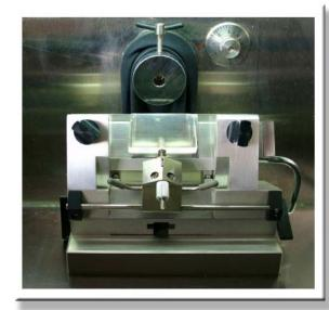
**Disposable blade holder** with adjustable cutting angle suitable with hall
